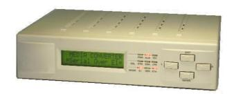
user with Ethernet over E1 conversion enabling the user to transport Ethernet data over an E1 link. It converts the Ethernet data into E1 frame format for transmission over the existing TDM (E1) links and then re-converts the E1 back into Ethernet data the far-end terminal. The device can effectively utilize the redundant bandwidth of telecom operators existing TDM network to transport Ethernet data with low investment. It can enable you to do as:
